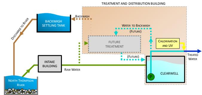
The proposed project engineered by TRUE Consulting will be made up of a raw water intake, an intake pumphouse, treatment (Phase 1 will include UV disinfection and chlorination, but does not include filtration) and a future treatment backwash.
